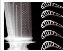
A 450 kV source in combination with a CLDA is ideal for radiographic and CT inspection as well as metrology of small to medium metal alloy turbine blades. Such an X-ray system offers sufficient source power to penetrate through the part and generate a scatter-free CT volume. In a production environment, the system runs
